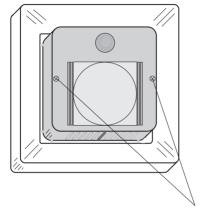
Reassemble the thermostat by first placing the frame, then mount the display module and finally press the front cover into place.
