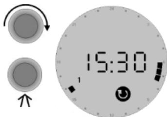
Then, turn until you reach the time when the next lowering of the temperature must start, e.g. 22:30, and press ...
