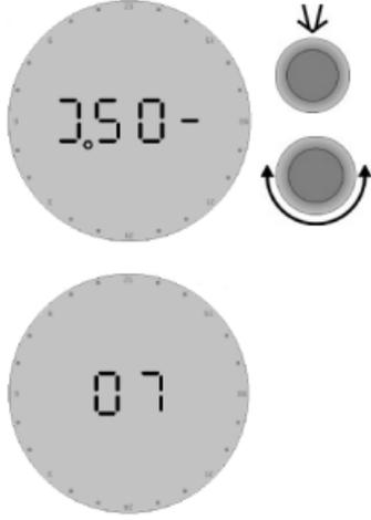
Offset (OFFS) can be used to adjust a variation between the thermostat and a thermometer in the room, if any. If the thermometer shows e.g. 1°C more than the thermostat, it is possible to adjust the offset with +1°C. The range is -5.5°C to +5.5°C.
